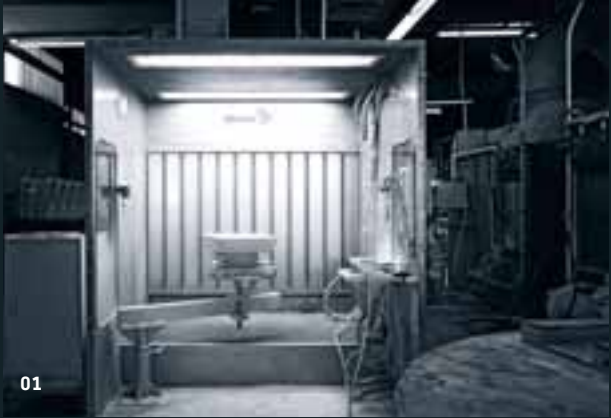
01-03 The enamel ensures a smooth surface that is easy to clean. At Duravit, it is exactly one millimeter thick. 04 Production in Meissen: after 21 hours in the kiln, the glaze of a toilet bowl is finished off. 05 Duravit test laboratories, like the one in Shanghai, really put our products through their paces in terms of functionality.
